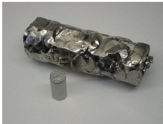
Figure 2.1. Zirconium crystal bar (Photo: W. Oelen in [4])
